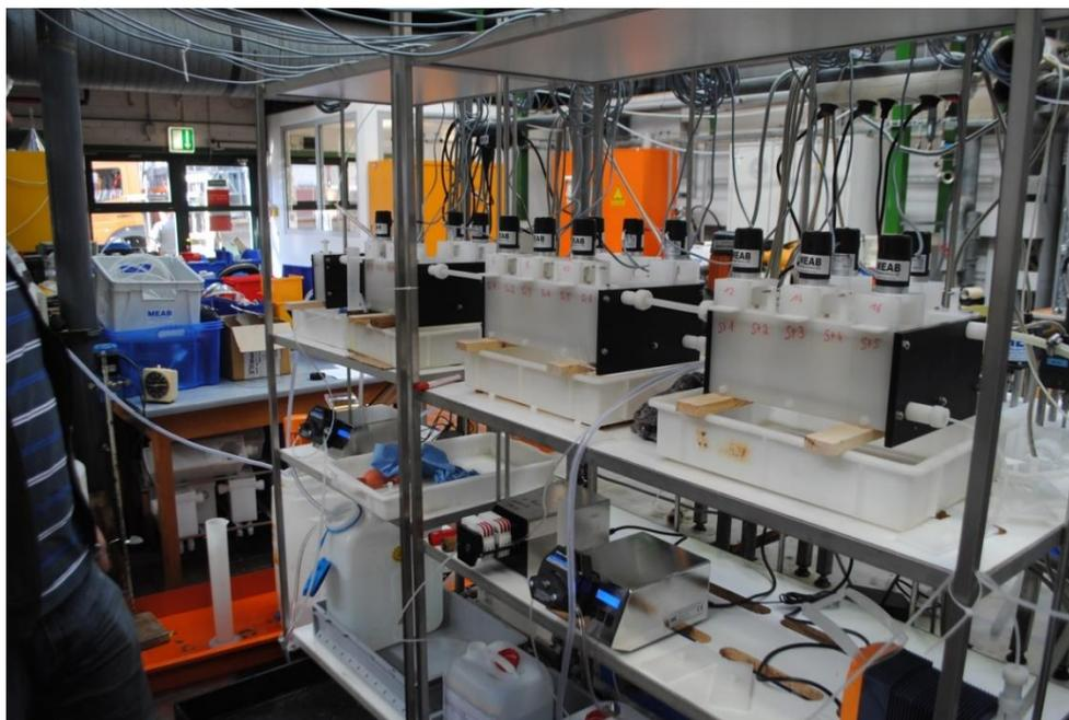
**Figure 3. MSU-0.5 multi stage laboratory unit for REE separation and purification**
